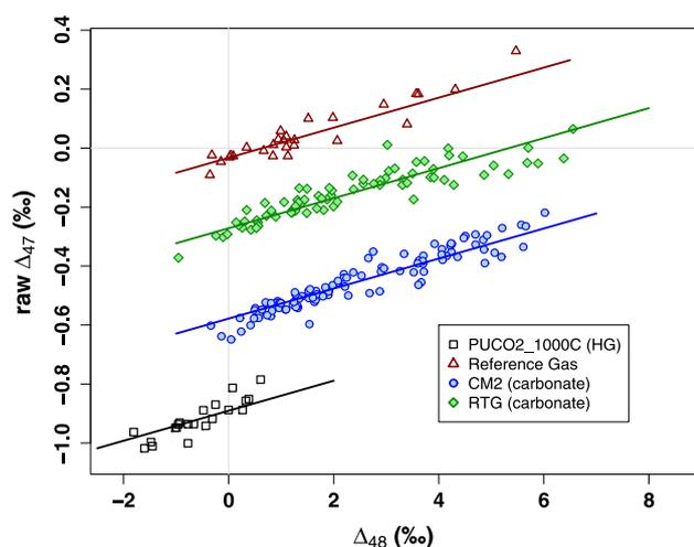
**Figure 4.** Correlation between  $\Delta_{48}$  and  $\Delta_{47\text{-raw}}$  shown for two carbonate standards, one heated gas, and the reference gas run as a sample, all run from September 2013 to March 2014. Lines are the result of a group regression to find a common slope (0.0509) and individual intercepts. Error bars are smaller than the symbols. Separate regressions of each sample type are found in Supplementary Table S1 (Supporting Information).
