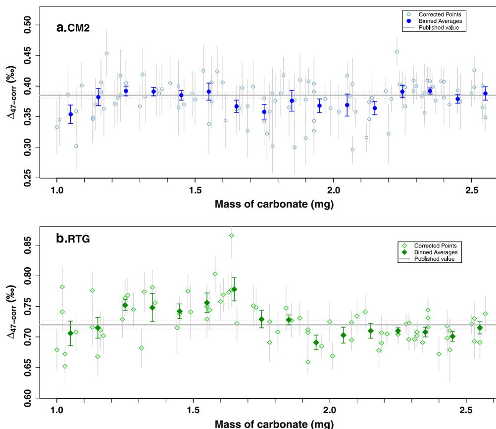
**Figure 6.** (a) Fully corrected  $\Delta_{47\text{-corr}}$  vs Mass for all CM2 points. Individual replicates are shown with error bars representing the original shot noise error fully propagated through all correction steps (see Supporting Information). Binned averages (0.1 mg bins) are shown in filled symbols. Grey horizontal lines indicate published value and error. (b) Same as (a) but for RTG.
