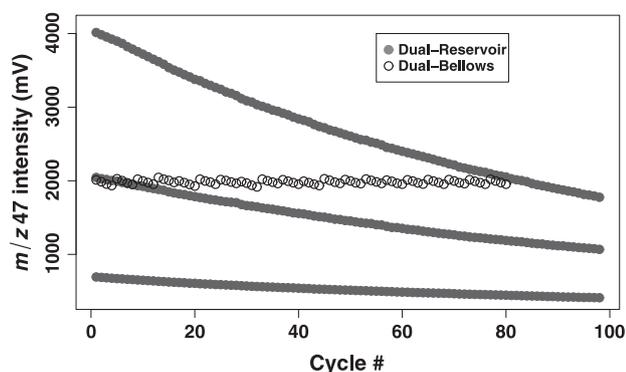
**Figure 2.**  $m/z$  47 beam intensity (mV) over the course of a sample run, shown for one run in the dual-bellows configuration (20 acquisitions  $\times$  4 cycles, target voltage 2 V on  $m/z$  47) and three runs in the dual-reservoir configuration with high, medium, and low starting voltages for  $m/z$  47 (7 acquisitions  $\times$  14 cycles, changing  $m/z$  47).  $m/z$  47 beam intensity decreases by 55%, 48%, and 41% for the three cases, respectively.
