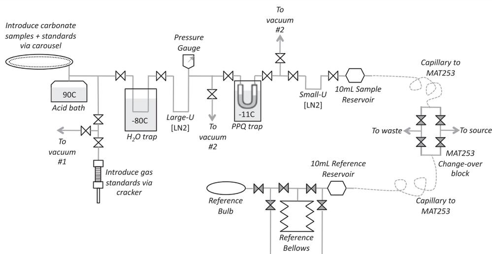
**Figure 1.** Diagram of the new, high-efficiency, dual-reservoir sample-preparation inlet. Double triangles represent valves. Shaded valves are controlled by the MAT 253, white valves are part of the inlet. Further details on where the 10 mL reservoir attaches to the mass spectrometer can be found in Supplementary Fig. S1 (Supporting Information).
