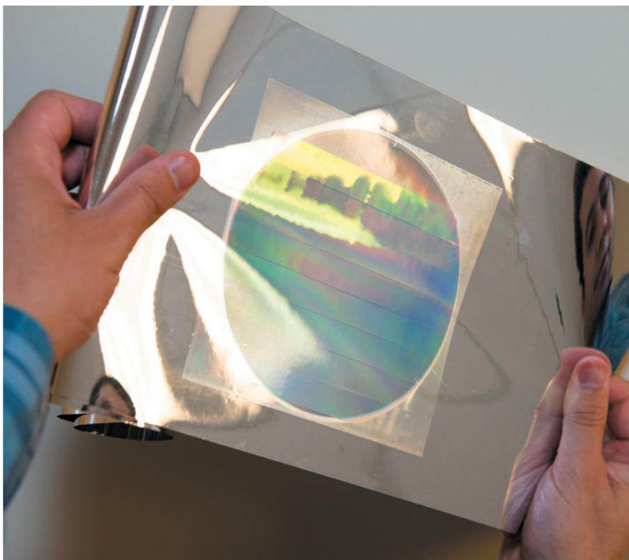
Ali Yetisen's printed holographic sensors can be used in wearable devices and textiles.
