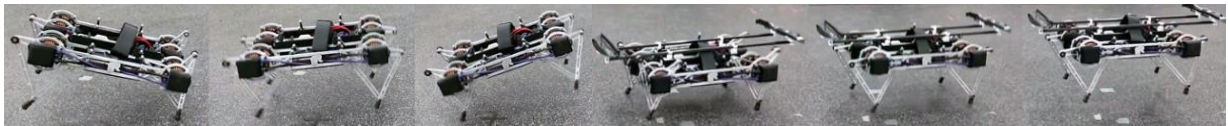
Figure 2: Preflexive bounding (left) and pronking (right) on Minitaur; stability of both are proved in (De and Koditschek, 2016).
