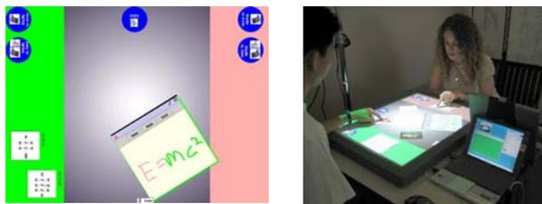
Figure 1. The UbiTable surface is divided into a center shared region, and two side, color-coded Personal Spaces. The circular icons are portals for moving documents to personal devices, and for copying. Each document on the table has a color border, indicating which user is using it, and a color bar on the top indicating ownership.
