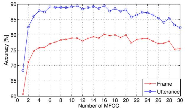
**Fig. 1.** Accuracy [%] for different number of MFCC.
