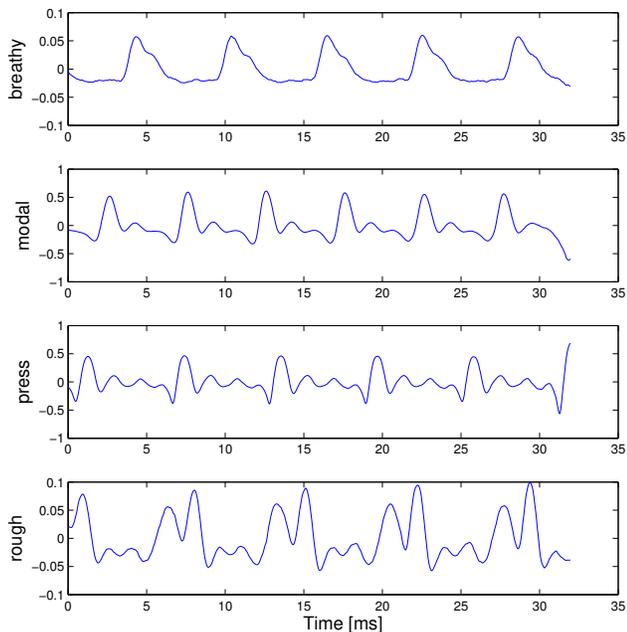
**Fig. 2.** Likelihood-averaged accelerometer waveforms for each voice mode.
