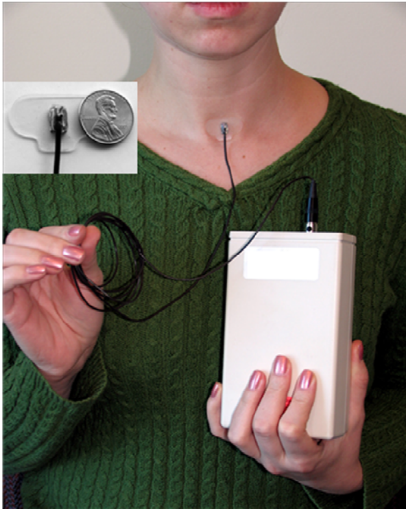
Figure 1. Illustration of the commercially-available APM Model 3200 worn by a speaker. The inset shows the size of the accelerometer (mounted on a soft silicone pad) relative to a US penny.
