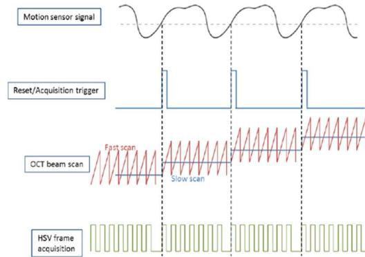
**Fig. 3.** OCT-HSV timing and synchronization diagram.
