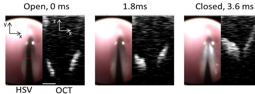
**Fig. 5.** Preliminary data displaying co-registered images acquired using swept-source OCT and HSV imaging modalities. The OCT beam scan path is indicated by a red dashed line. Scale bar: 1 mm.
