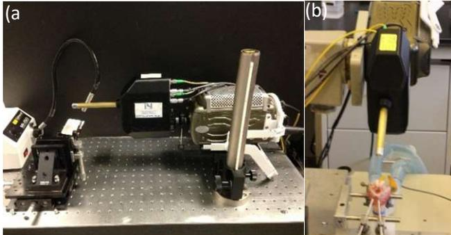
**Fig. 2.** OCT-HSV instrument. Setup showing (a) the OCT probe head mounted on the high-speed camera for co-linear imaging through a rigid endoscope and (b) the ex vivo calf larynx being imaged.
