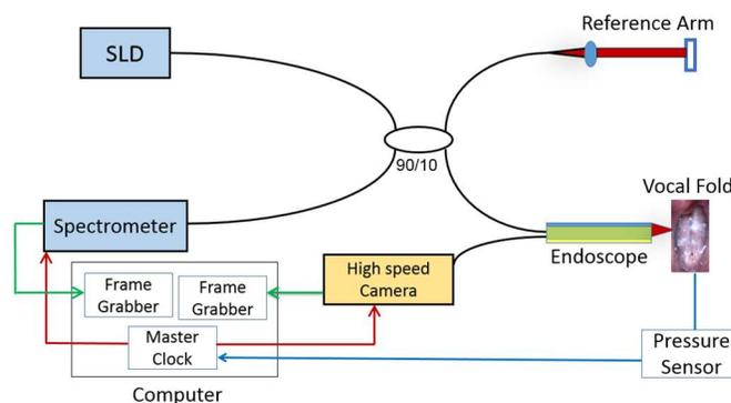
Fig. 1. Schematic of the integrated OCT-HSV instrument.
