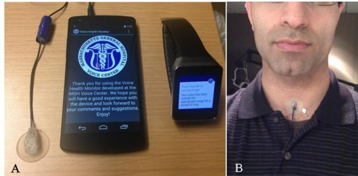
Figure 1. Smartphone-based ambulatory voice monitor: (A) accelerometer, interface cable, smartphone, smartwatch; (B) accelerometer mounted on a silicone pad affixed to the neck above the collarbone.
