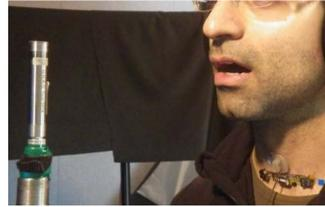
**Four adult participants** (two male, two female) wore the wireless voice monitor inside an acoustically treated sound booth that contained loudspeakers that allowed for the **simulation of ambient acoustic stimuli** at varying calibrated sound pressure levels. Each participant performed the following speech tasks:
