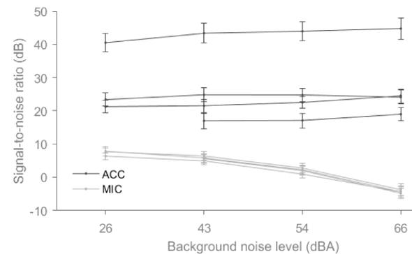
**Comparison of signal-to-noise ratio (SNR) of the ACC and MIC signals** for the Rainbow Passage. Error bars:  $\pm 1$  std. dev.
