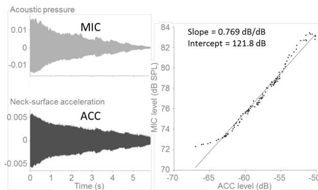
**Participant-specific calibration** of accelerometer (ACC) signal level to microphone (MIC) sound pressure level using the loud-to-soft vowel task.
