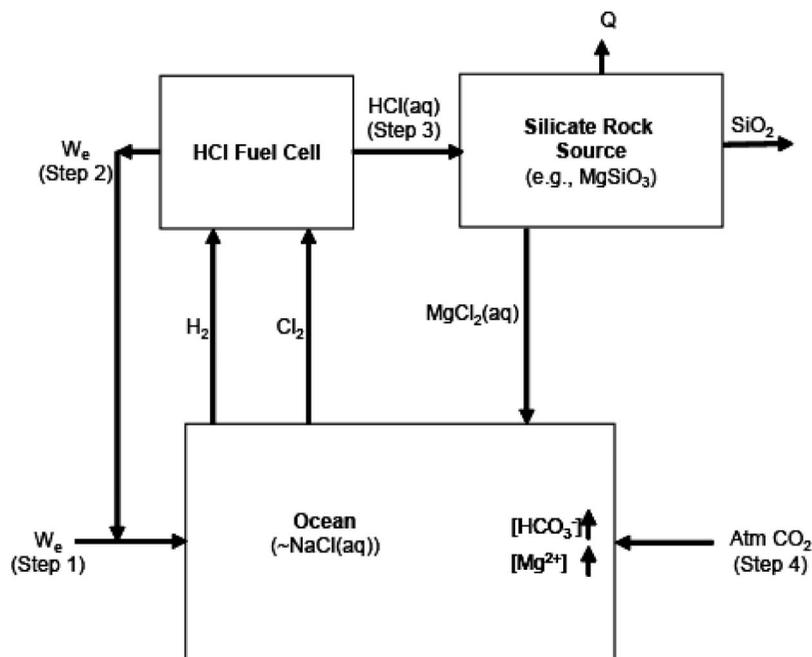
**FIGURE 1.** Diagram showing carbon dioxide sequestration via the removal and neutralization of hydrochloric acid from the ocean. Magnesium has been used to represent any metal found in silicate rocks.  $W_e$  represents electrical work and  $Q$  represents heat.
