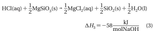
For every mole of NaOH produced in Step 1, the dissolution of enstatite will generate  $\sim 58$  kJ of heat. The kinetics of rock dissolution are an important consideration for this process, and the kinetics of silicate rock dissolution are highly dependent on pH and temperature (18).
