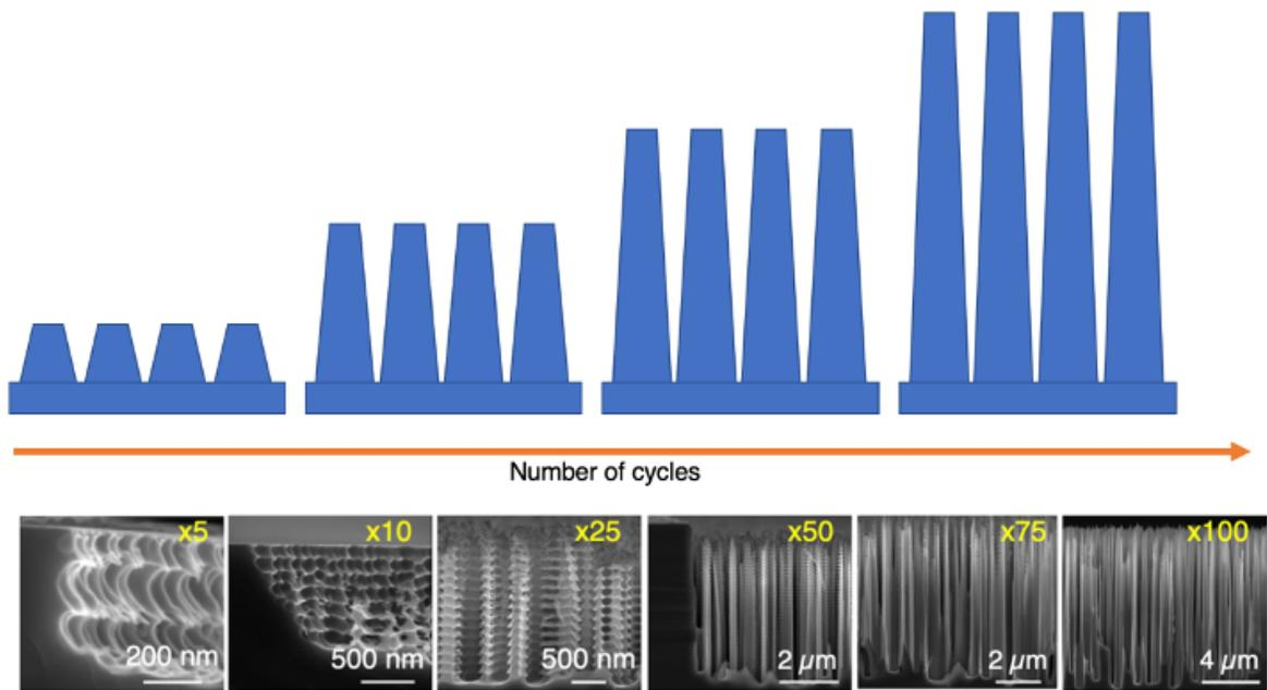
Figure 3: Expected nanopillar structures. SEM images are sourced from [4]. Note that meaningful nanostructures start emerging with >10 cycles.
