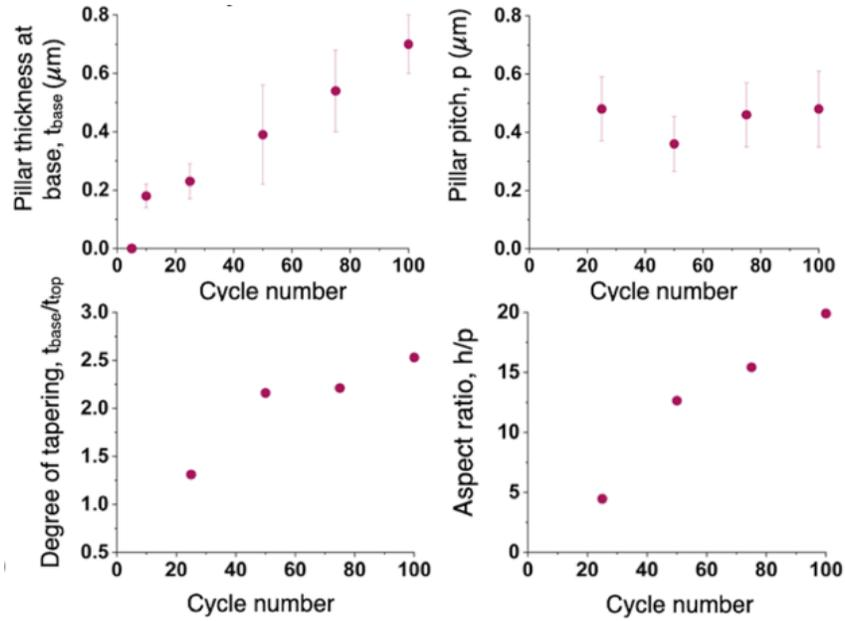
Figure 2: Demonstrates linear increase in aspect ratio and pillar thickness with number of etch cycles. [4]
