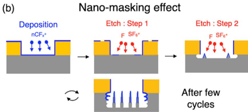
Figure 1: For the given etch process parameters, the etch process is strong enough to remove the deposited polymer at flat surfaces, but not at high aspect ratio structures. The result is a reproducible nano-pillar structure with increasing pillar height and approximately constant pillar thickness, formed without a lithography process. Figure adapted from [4].
