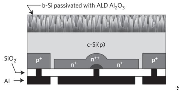
Figure 4: Example b-Si solar cell
