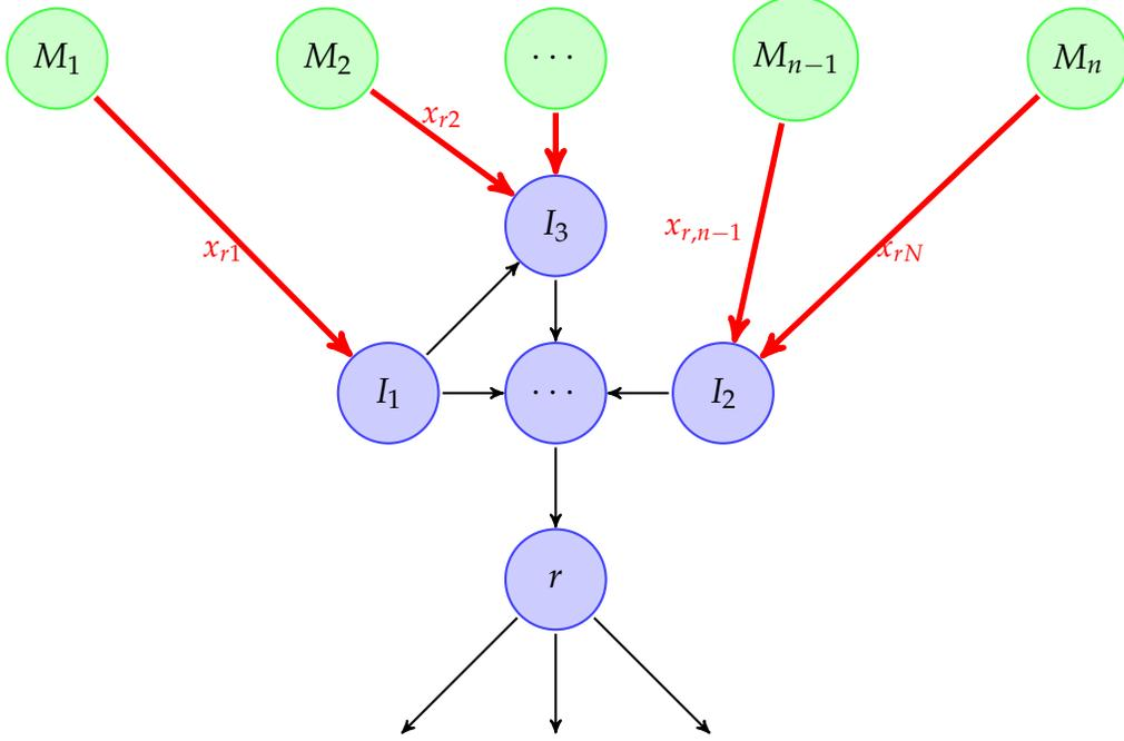
Figure 1: Illustration of an island  $(r, I, M)$  within a broader network. The nodes in the island  $I$  are in blue, the imports  $M$  are in green, and the export of the island is denoted by  $r$ . The figure only shows the island, its imports, and its export. This island is embedded in a broader network which is not explicitly represented in the figure.
