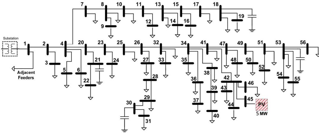
Fig. 1: Schematic diagram of the SCE distribution systems.
