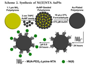
slightly from bright to dark yellow, and TEM images display the THPC-functionalized AuNP seeds adsorbed to the surface of the amine-terminated microspheres (Figure 1A,B). AuNP-
