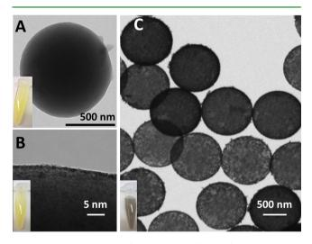
Figure 1. Characterization of AuPSs upon addition of AuNP seeds and Au plating. TEM images of (A) an amine-terminated polystyrene sphere, (B) the surface of a polystyrene sphere with adsorbed 2-4 nm AuNPs, and (C) Au-plated polystyrene spheres (AuPSs). The insets at the bottom left of each panel show the color of a 1 pM aliquot of each type of microsphere.
