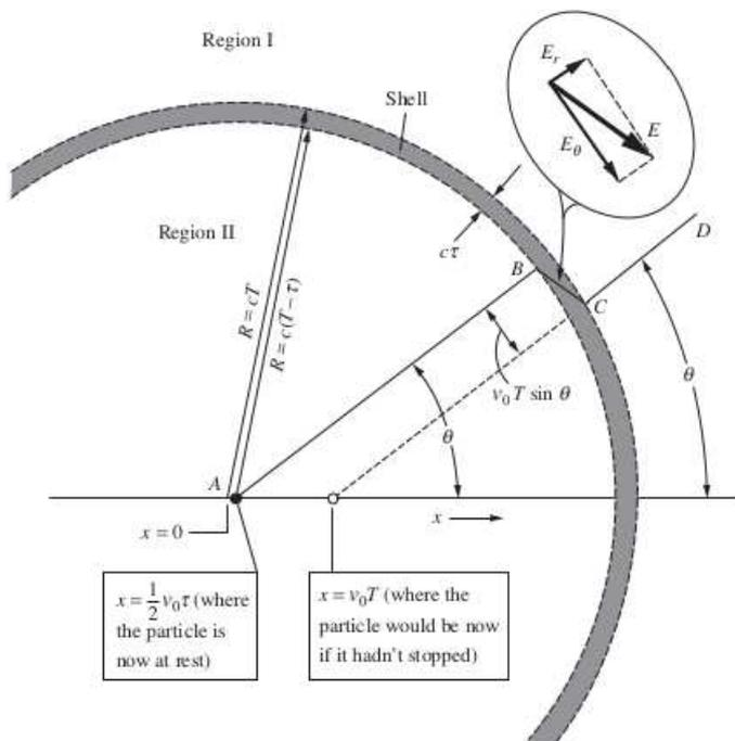
**Figure H.2.** Space diagram for the instant  $t = T \gg \tau$ , a long time after the particle has stopped. For observers in region I, the field must be that of a charge located at the position  $x = v_0 T$ ; for observers in region II, it is that of a particle at rest close to the origin. The transition region is a shell of thickness  $c\tau$ .
