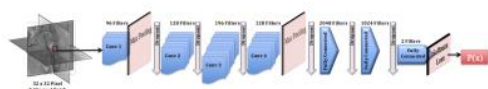
Figure 1: Network Architecture - A combination of convolutional, max pooling, dropout, fully connected, and loss layers were used to generate probability output at the voxel of interest location. Stochastic gradient descent with momentum was utilized to back-propagate through network during learning.
