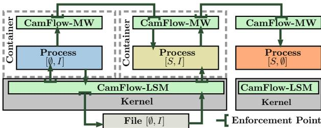
Fig. 5: High-level view of CamFlow use for PaaS.
