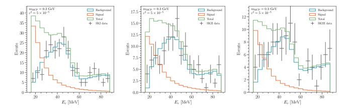
FIG. 10. Distributions for our millicharged particle search for the three stages of Super-Kamiokande. Data is shown as crosses and expected background is shown as a blue histogram. An example millicharge particle distribution is shown, for the same parameters, as an orange histogram.
