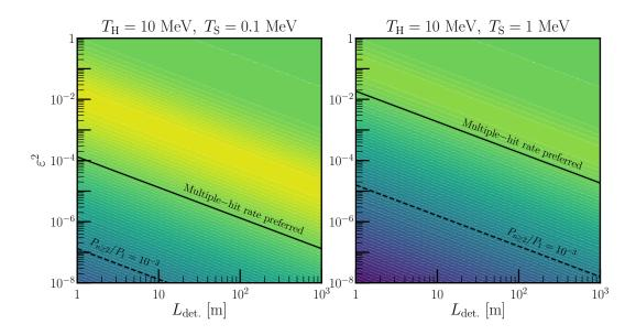
FIG. 8. Multiple-hit vs. single-hit search ratios. Ratio of multiple soft-scatter events to single hard-scatter events as a function of total detector length  $L_{\text{det.}}$  and  $\varepsilon^2$  for two choices of  $T_{\text{H}}$  and  $T_{\text{S}}$ , as labelled. Above the solid black lines, the double-hit rate exceeds the single-hit one. Above the dashed lines, the double-hit rate is at most three orders of magnitude smaller than the single-hit one.
