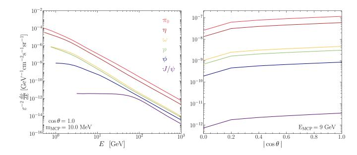
FIG. 2. Flux of millicharged particles from different parent mesons. Left: Spectra, which scales as  $\varepsilon^2$ , of millicharged particles arriving at the surface of the Earth with zenith angle 0°, for each one of the different parent mesons. Right: Angular dependence of the flux at 9 GeV. In both panels the MCP mass is set to 10 MeV.
