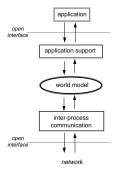
Figure 2: Internal structure of a Spline process.
