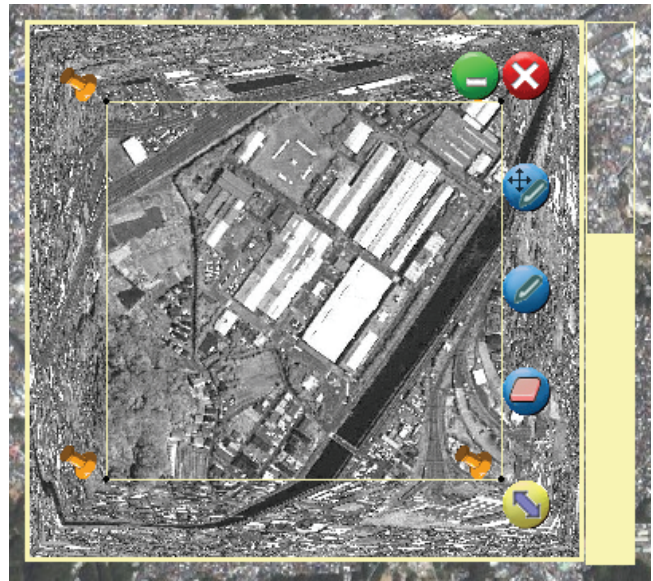
Figure 3. When locked into place, a lens displays controls for minimizing, closing, annotation, resizing, and for changing the magnification.
