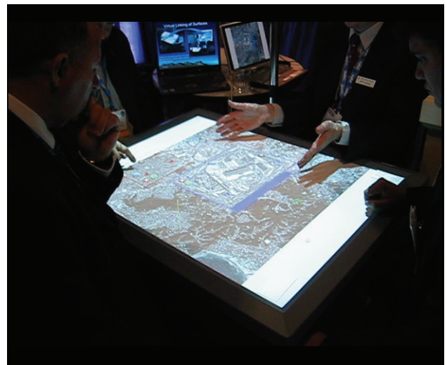
Figure 1. A group of people sitting around the table using DTLens to view multiple portions of a 7300 x 5400 pixels image simultaneously.
