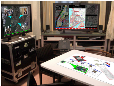
Figure 10a. The emergency management scenario: an interactive table augmented with two large displays (enhanced photograph). Figures 10b-d show details.
