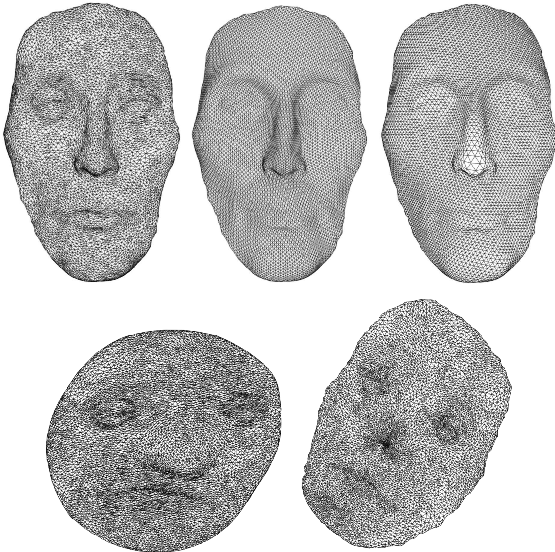
Figure 23. Remeshing a human face. Top left: the original human face. Top middle: the remeshing result via our parameterization. Top right: the remeshing result via the free-boundary conformal parameterization by Desbrun, Meyer, and Alliez [19]. Bottom left: the density-equalizing parameterization by our algorithm. Bottom right: the free-boundary conformal parameterization by Desbrun, Meyer, and Alliez [19].
