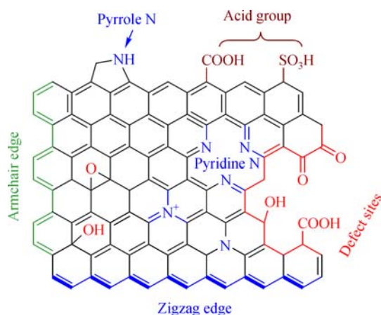
Fig. 2 Schematic diagram of active sites of graphene derivatives
