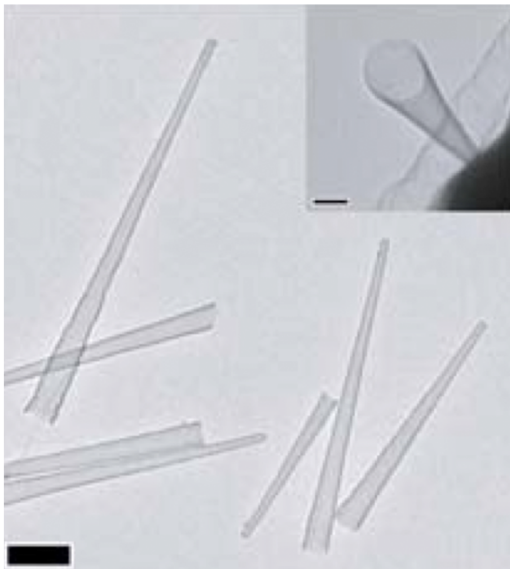
Figure 5.8: Nanocones templated from highly tapered Ge cores grown at 380°C. Scale bar is 200 nm. Inset: The base of a typical cone, viewed at an oblique angle, is round and hollow (scale bar, 200 nm).
