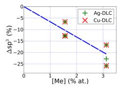
FIG. 2. Change in the sp<sup>3</sup>-bonded C,  $\Delta$ sp<sup>3</sup>, as a function of the metal concentration [Me] in Ag- (green) and Cu- (red) containing DLC. The slope of the approximate linear fit to the results corresponds to 6.9% decrease in sp<sup>3</sup>-bonded C for 1% increase in metal content.
