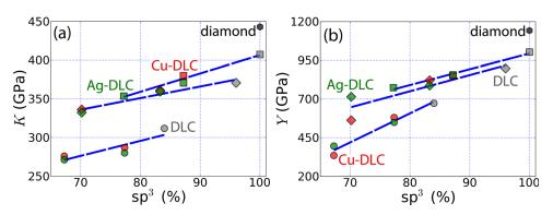
FIG. 5. (a) Bulk *K* and (b) Young's *Y* modulus of metal-free (gray), and Agred) and Cu- (green) containing DLC. Different symbols mark different content in sp<sup>3</sup>-bonded C in the unmodified (metal-free) DLC. A linear relationship describes the correlation between the content in sp<sup>3</sup>-bonded C and the elastic moduli
