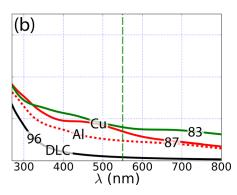
FIG. 4. Absorption coefficient  $\alpha$  for metal-free (black line), and Al- (dashed line), Cu- and Ag- (solid lines) containing DLC. Different colors correspond to different content in sp<sup>3</sup>-bonded C (indicated as percentage on top of each family of curves) and metal. The peak of the solar spectrum ( $\lambda = 550\,\mathrm{nm}$ ) is marked with a vertical green, dashed line.
