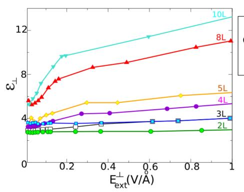
The dielectric constant of graphene is electric-field dependent
