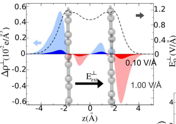
Charge accumulation/depletion at graphene layer generates the response field.
