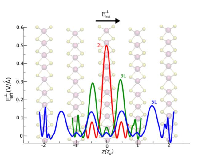
The electric field inside of the material decreases as a function of the number of layers.
