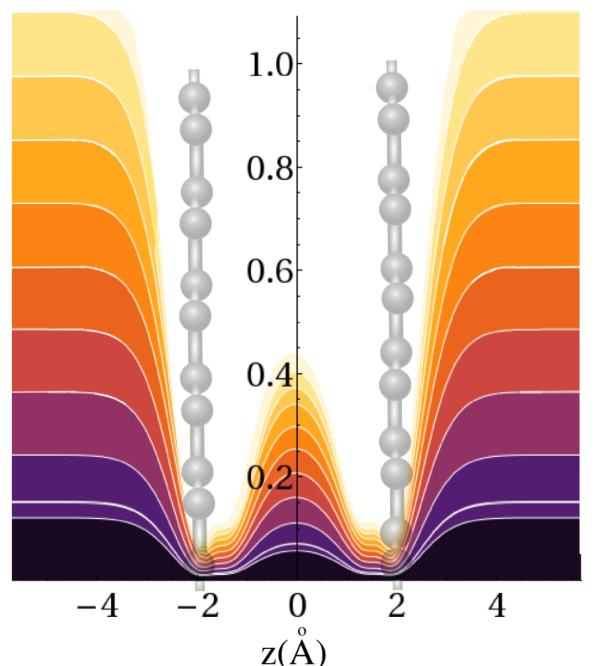
Position-dependent interlayer electric field (maximum and minimal values)
