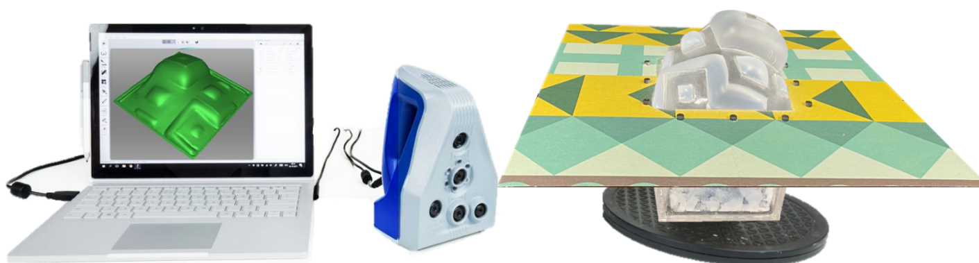
Figure 10: Artec Space Spider 3D scanner acquisition set up.
