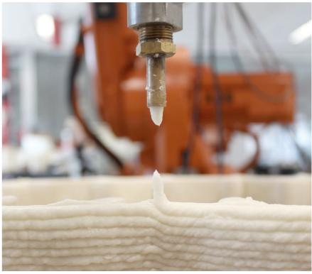
session gave its place to understanding how to segment for improved throughput: as the process is not bottlenecked by thermo-dispensing such as in large diameter FDM, printing can be much faster, for example 50mm/sec at 7mm diameter, while curing takes place separately. It became evident that it was thus more meaningful to consider scaling in terms of time, within a heterogenous sequence of production steps, instead of targeting physical scale using additive manufacturing exclusively.
