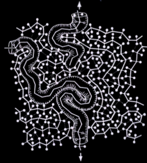
Fig. 23.4. Each molecule in a linear polymer can be thought of as being contained in a tube made up by its surroundings. When the polymer is loaded at or above T_g , each molecule can move (reptate) in its tube, giving strain.
