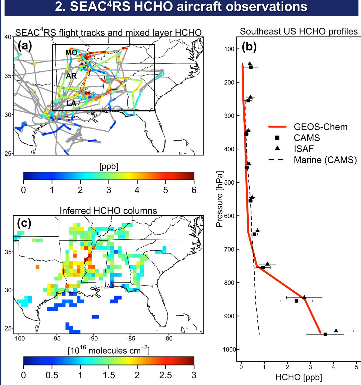
(a) SEAC<sup>4</sup>RS DC-8 flight tracks (in grey) and the CAMS measurements aboard the aircraft in the mixed layer. (b) Mean vertical profiles observed by the CAMS and ISAF instruments, and simulated by GEOS-Chem, for the Southeast US domain (box in panel a). (c) Mean HCHO columns derived from the CAMS.
