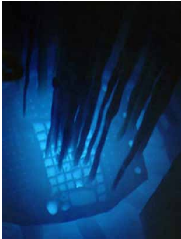
Thorium-uranium fuel assemblies being tested at the Kurchatov Institute in a joint Russian-American project could reduce nuclear waste and make spent fuel more proliferation resistant – a good example of the potential for U.S.-Russian cooperation in nuclear energy research and development.
