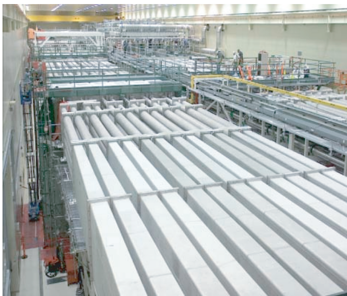
Figure 14.24 | Laser beam lines at the National Ignition Facility at Livermore National Laboratory, California. Source: FESAC, 2003.
