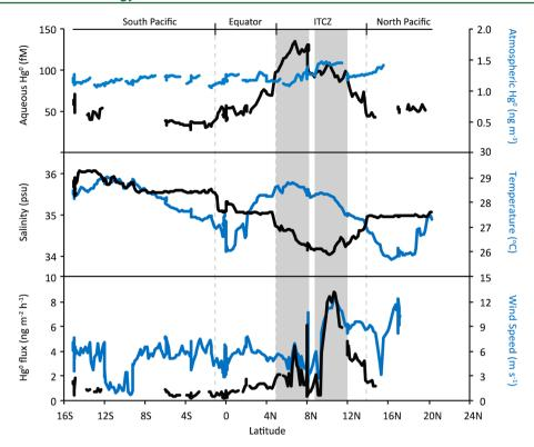
**Figure 2.** Latitudinal variability in measured atmospheric and seawater  $Hg^0$  concentrations, associated evasion, and environmental properties on the METZYME cruise. Shaded areas denote statistically different regions for  $Hg^0$  concentrations within the region reflecting the ITCZ.
