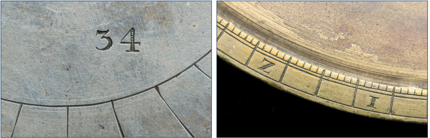
Fig. 3 Detail of engraving style on (left) tympan and (right) mater of Harvard's DW0594 showing the unusual infill of some of the broad strokes. Courtesy of the Collection of Historical Scientific Instruments, Harvard University.
