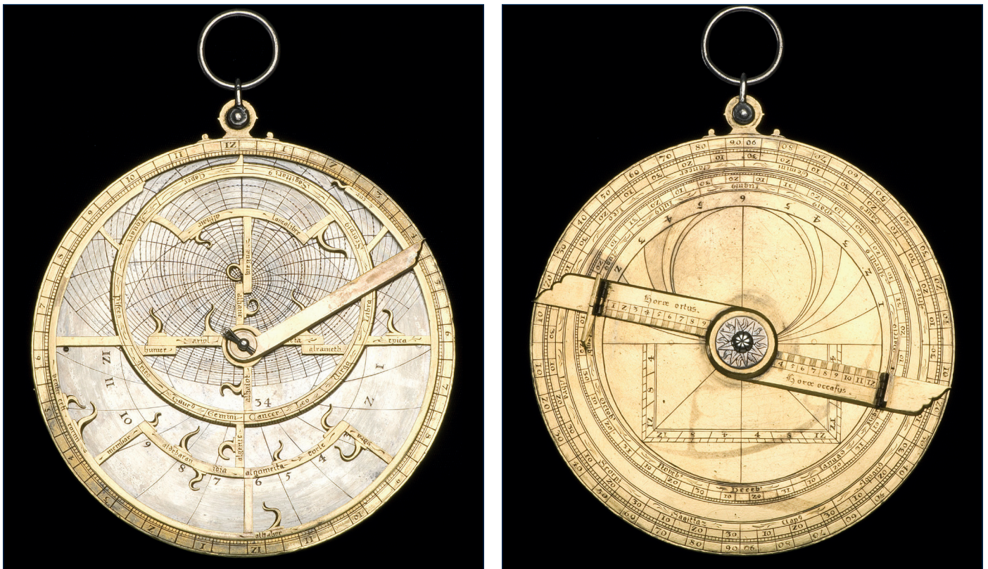
Fig. 1 Fusoris-style planispheric astrolabe at Harvard, inv. no. DW0594, (left) front and (right) back views. Courtesy of the Collection of Historical Scientific Instruments, Harvard University.
