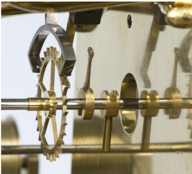
A view of the movement between the plates of an astronomical regulator by Simon Willard Jr., Boston, 1832. It shows the Graham deadbeat escapement with jeweled pallets. To the right of the escape wheel on the same arbor is the break-circuitry contact finger and its counter balance. (The other end of the contact has been moved out of the way, because it is not being used.) (Collection of Historical Scientific Instruments, Harvard University, inv. no. 2500)
