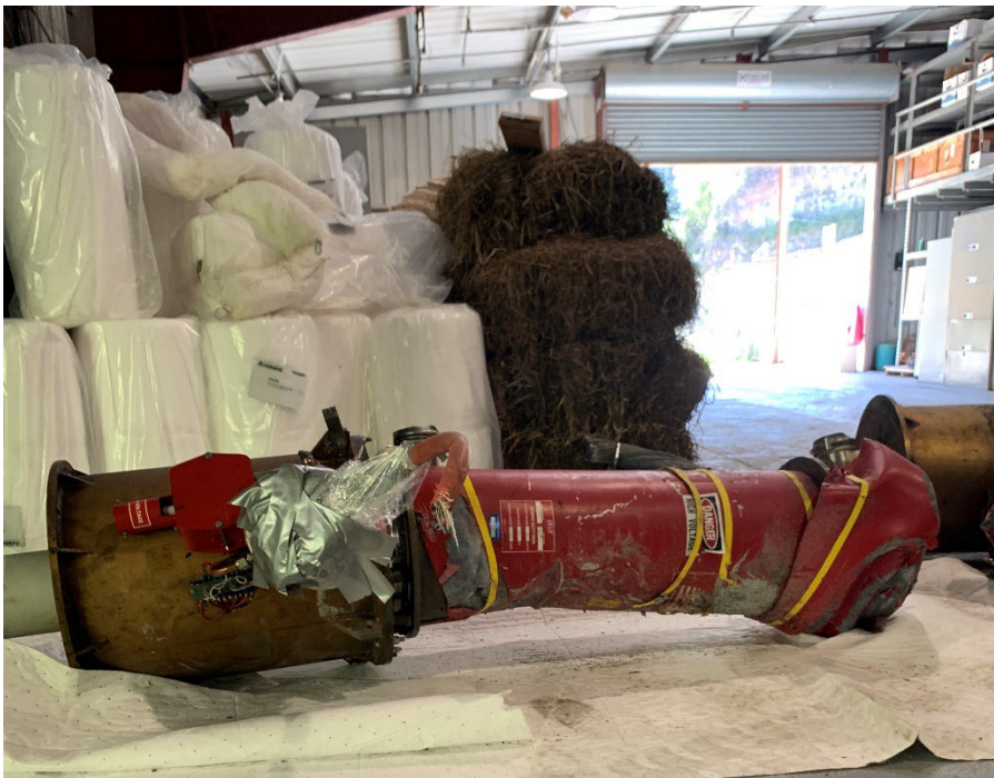
Figure 3. Planetary Radar S-band Klystron (2380 MHz, 12 cm, 500 kw). These instruments were among the key elements for Planetary Sciences research especially on Near-Earth Objects, Main Belt Asteroids, comets, and neighboring planets
