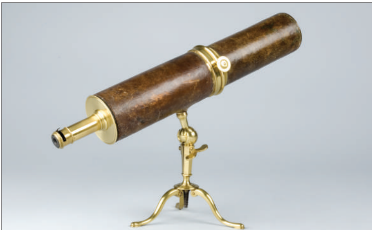
Fig. 2 - Gregorian reflecting telescope, English, circa 1735, owned by astronomer, John Winthrop, Hollis Professor of Mathematics and Natural Philosophy, Harvard College. Collection of Historical Scientific Instruments, Harvard University, 0054.
