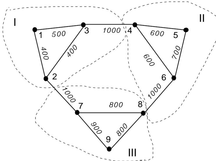
*Thermal limits on transmission lines (MW).*
