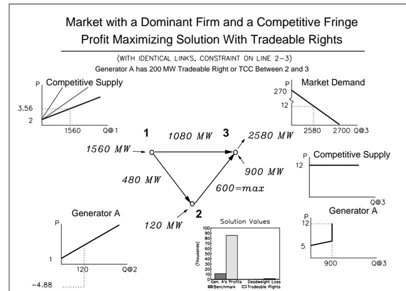
The case here differs J&T in that the monopolist controls generation at more than one location, and some of its generation is low cost. The details show financial contracts increase efficiency in this case.<sup>1</sup>
