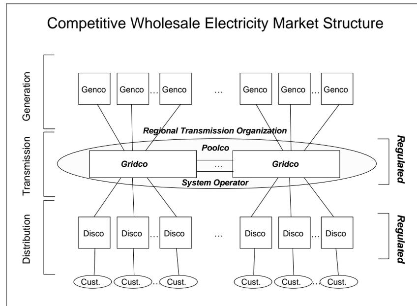
The special conditions in the electricity system stand as barriers to an efficient, large-scale bilateral market in electricity. A pool-based market model for regional coordination helps overcome these barriers.
