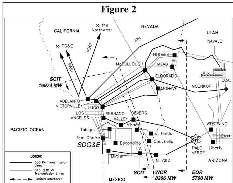
The map provided by San Diego Gas & Electric (SDG&E) illustrates the location of major power plants, loads, and transmission lines. The schematic includes three interfaces with associated maximum transfer limits: The East of River (EOR) with a maximum of 5700 MW, West of River (WOR) with a maximum of 8206 MW, and the Southern California Import Transmission
